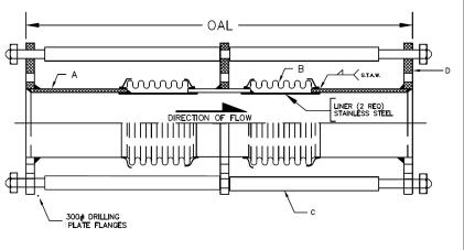
AXIAL MOVEMENT RATED AT 1.6" AND 0.4" EXTENSION DESIGN PRESSURE = 300 PSIG @ 70°F
