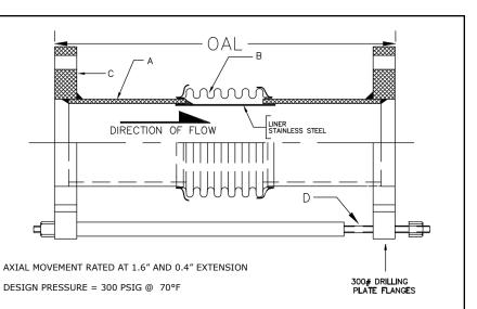
308 SERIES EXPANSION JOINT 2" TRAVEL W/300# PLATE FLANGES & TIE RODS
