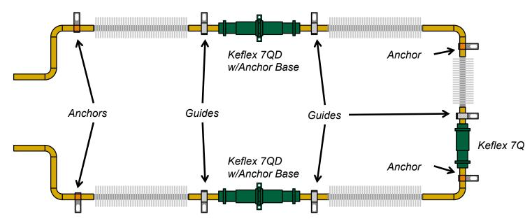
Expansion compensators must be both correctly selected and properly installed for effective performance in service. The reactions created by pressure and movement within the piping system should be carefully considered and the following precautions taken at installation:
