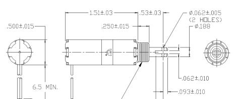
3/8-32 UNEF-2A THREAD Solenoid shown energized with plunger fully seated Supplied with mounting bracket, hex nut and lock washer shipped loose
