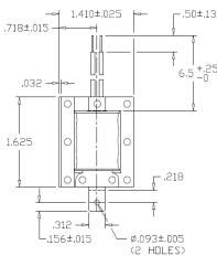
Solenoid shown energized with plunger fully seated
