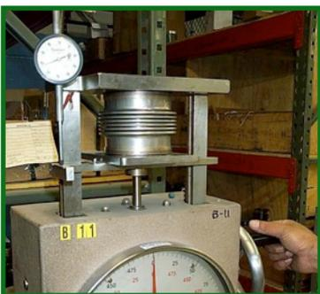
**LOWER THRUST FORCES** - The multi-ply design results in lower spring rates. Also, the effective cross sectional area of multi-ply expansion joints is less, compared to single-ply bellows, to accommodate a given movement. These two reductions result in lower forces and moments on the anchors, equipment and guides. A side benefit is that less anchors and guides will be required in the overall bellows piping system.
