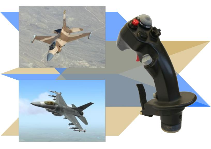
Designed for the F-16 Falcon, this grip has widened its appeal among manufacturers and is becoming the choice for retrofits and upgrade packages. Equipped with a large 4- way switch, six pushbutton or mini 4-way switches, a trigger, and an autopilot override fingertip lever, the F-16 grip elevated Hands On Throttle-And-Stick (HOTAS) systems to the next level. This is one of the few grips designed for side- arm control in the cockpit, as compared to between-the-leg controls.
