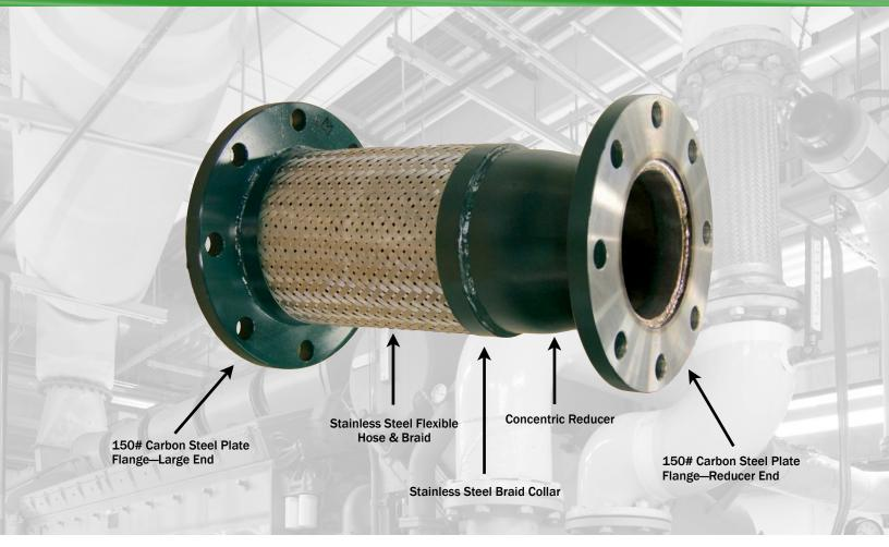
KEFLEX™ Gold Series Reducing braided flexible hose assemblies are constructed of stainless steel annular corrugated metal hose surrounded with a woven braid of high tensile stainless steel. The KEFLEX™ Gold Series is the premier product in the industry.
