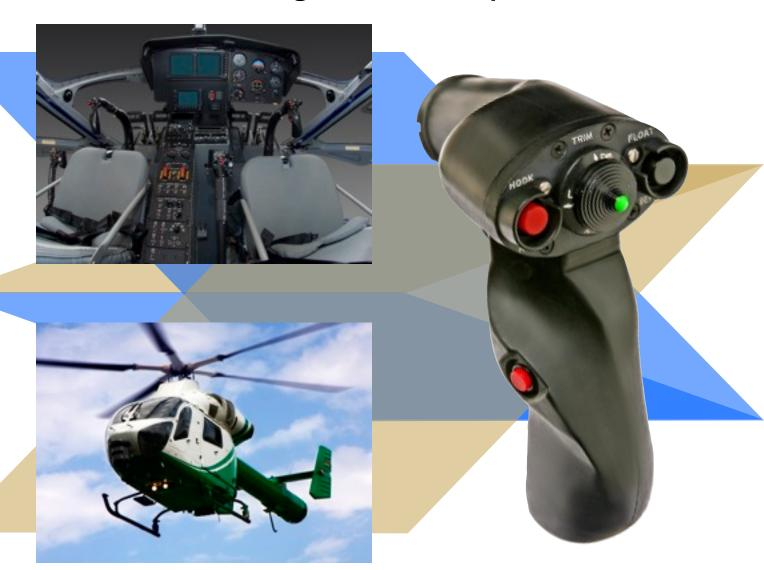
The MD Standard control grip keeps vital flight functions at the pilot's fingertips. The large central 4-way switch trims up the helicopter for stability in flight and hover modes. Pushbuttons control the hook release (for slung loads) and float deployment (for naval operations). The trigger switch changes frequencies between on-board intercom systems and group-wide radio transmissions. The thumb-rest switch typically engages landing lights or spotlights.
