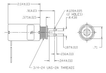
Solenoid shown energized with plunger fully seated Supplied with mounting bracket, hex nut and lock washer shipped loose
