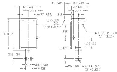
Solenoid shown energized with plunger fully seated
