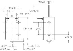
Solenoid shown energized with plunger fully seated in extended position
