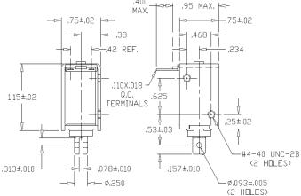
Solenoid shown energized with plunger fully seated
