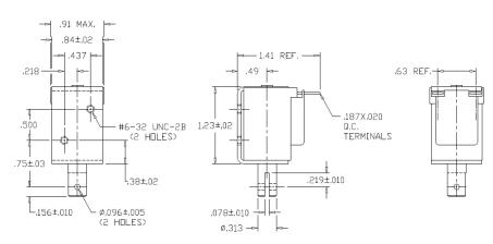
Solenoid shown energized with plunger fully seated
