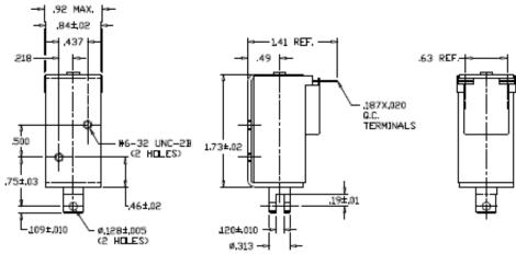
Solenoid shown energized with plunger fully seated
