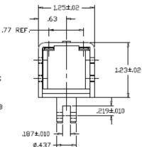
Solenoid shown energized with plunger fully seated
