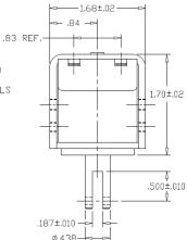
Solenoid shown energized with plunger fully seated
