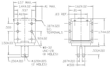
Solenoid shown energized with plunger fully seated
