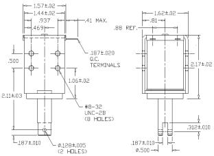
Solenoid shown energized with plunger fully seated
