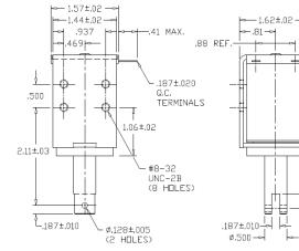
Solenoid shown energized with plunger fully seated
