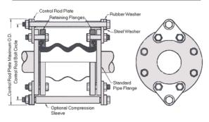
Technical Note: Flex-Weld strongly encourages the use of Control Rods in most, if not all, Rubber EJ applications. Most applications that utilize rubber expansion joints are not anchored properly. A simple pump connector does not protect against extreme stresses and strains produced by water hammer or air induced surge pressure, common to most applications, which greatly exceed normal system operating pressure.
