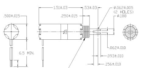
Solenoid shown energized with plunger fully seated Supplied with mounting bracket, hex nut and lock washer shipped loose
